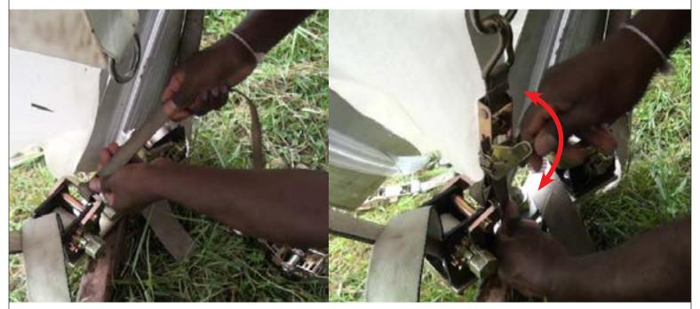
5 Tighten each side evenly and ensure that seam is at Center
